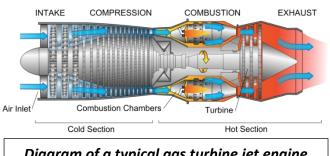
Diagram of a typical gas turbine jet engine (Jeff Dahl 2007)
