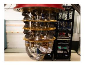
Google declared 'Quantum Supremacy' in the Nature journal on the 23rd October 2019 which essentially means that their Sycamore processor has experimentally proved that Quantum computers have been shown to solve and run problems at a much faster rate than classical computers. While Sycamore (the name of the computer) had 54 qubits, only 53 worked during the experiment.
