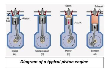
To understand why the jet engine was such a huge leap forward, first we need to get a sense of what flying was like before it. Up until the 1940s, planes were powered by internal combustion piston engines, which are essentially the same type of engines found in cars. Piston engines simply cannot be as powerful as jet engines in the way that they work, despite using the same scientific principles as jets with the same four stages of intake, compression, combustion and exhaust.
