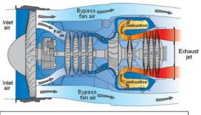
Diagram of a turbofan engine
