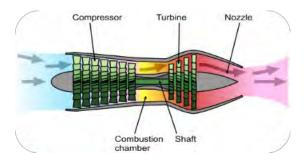
Figure 2 A turbojet engine
