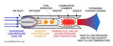
Figure 3 A ramjet engine
