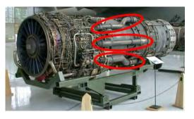
Figure 8 Bypass tubes on a J58
