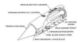
Figure 12 Key parts of the forward section of the nacelle
