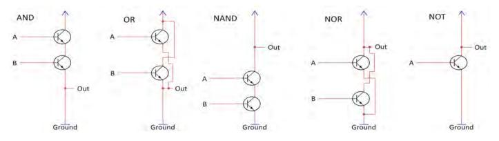
Figure 1 - Transistors used to make logic gates
