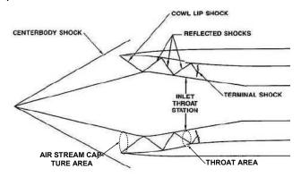
Figure 10 Shockwaves formed in the inlet
