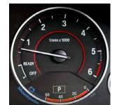
Tachometer on a BMW, with redline between 5500 RPM and 6000 RPM
